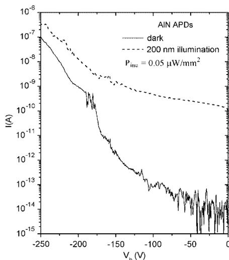
FIG. 2. Reverse  $I$ - $V$  characteristics of  $d=100 \mu\text{m}$  diameter AlN APDs in dark and under 200 nm light illumination. The incident power density at 200 nm is  $0.05 \mu\text{W}/\text{mm}^2$ .
