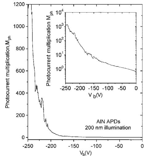
FIG. 3. Photocurrent multiplication or gain of an AlN APD with  $d=100 \mu\text{m}$   $M_{\text{ph}}$  as a function of the reverse bias voltage  $V_b$ .  $M_{\text{ph}}$  increases only slowly at  $|V_b| < 180$  V, but increases exponentially at  $|V_b| > 180$  V and reaches about 1200 at  $V_b=-250$  V. The inset is the same plot in the semilog scale.
