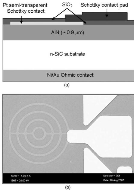
FIG. 1. (a) Schematic layer structure of AlN APDs and (b) SEM image of a fabricated AlN APD with  $d=100 \mu\text{m}$  in diameter.
