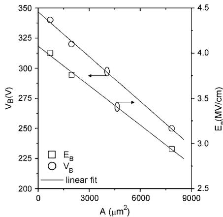
FIG. 5. Reverse breakdown voltage ( $V_B$ ) and breakdown field ( $E_B$ ) as functions of the device area  $A(=\pi d^2/4)$  for AlN APDs. The solid lines are the linear least square fits of data. The breakdown field of dislocation-free AlN epilayer ( $E_B$  at  $d=0$ ) is about 4.1 MV/cm.
