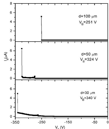
FIG. 4. Reverse bias  $I$ - $V$  characteristics of AlN APDs with  $d=100, 50,$  and  $30 \mu\text{m}$  in diameter. The breakdown voltage  $V_B$  increases with decreasing device size.
